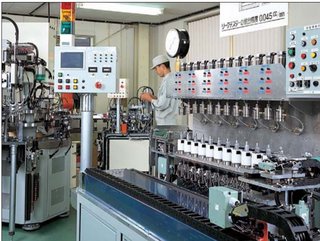
▲ Automatic coupling inspection equipment
