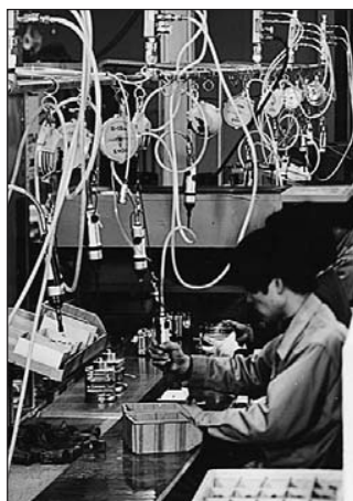
▲ Air pipe branching
