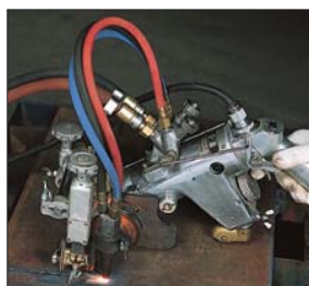
▲ For piping for welding / cutting equipment
