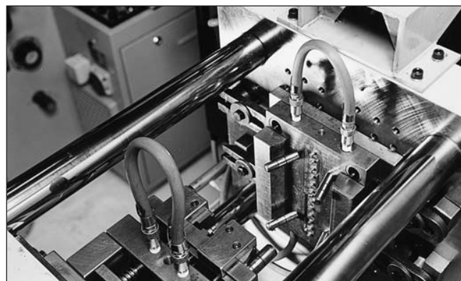
▲ Mold coolant hoses
